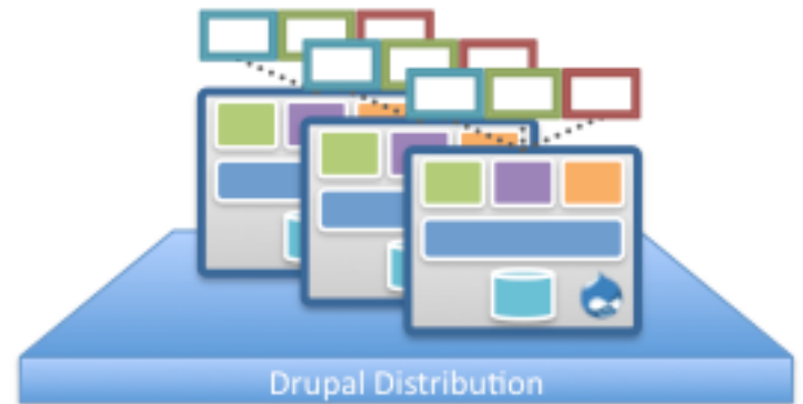
Illustration 3. With a hybrid configuration, a single Drupal distribution spawns an extensible set of Drupal-powered websites. All sites have the same set of modules and their own website databases.
